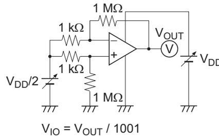
7. Input Offset Voltage,  $V_{IO}$
