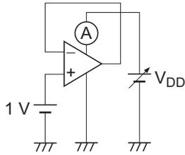
2. Output High Voltage,  $V_{OH}$  (Output High)
