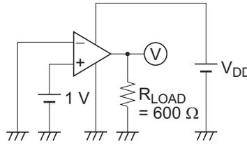
3. Output Low Voltage,  $V_{OL}$  (Output Low)
