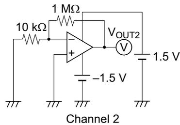
$$CS = \left| 20 \log_{10} \frac{101 \times |V_{OUT2}|}{|V_{OUT1}|} \right|$$
