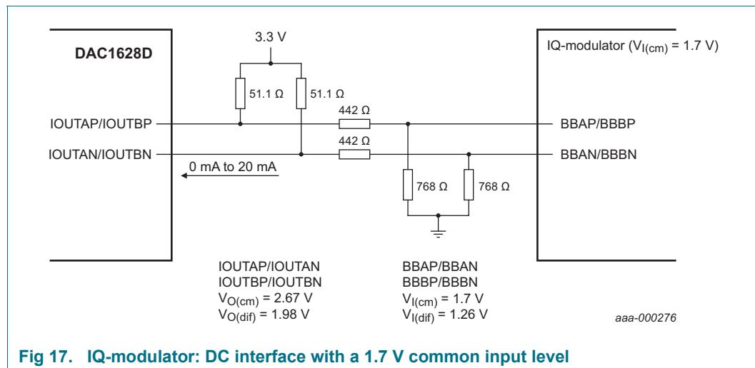
**Fig 17. IQ-modulator: DC interface with a 1.7 V common input level**
