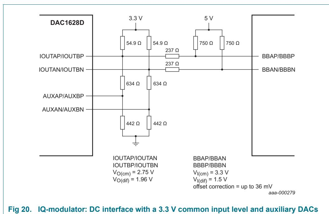
**Fig 20. IQ-modulator: DC interface with a 3.3 V common input level and auxiliary DACs**
