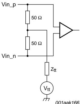
**Fig 4. Lane input termination**
