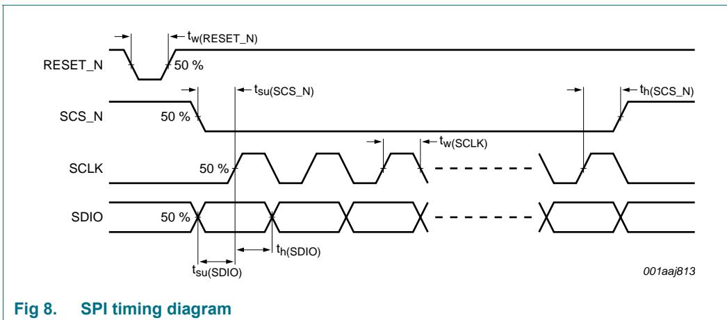
Fig 8. SPI timing diagram
