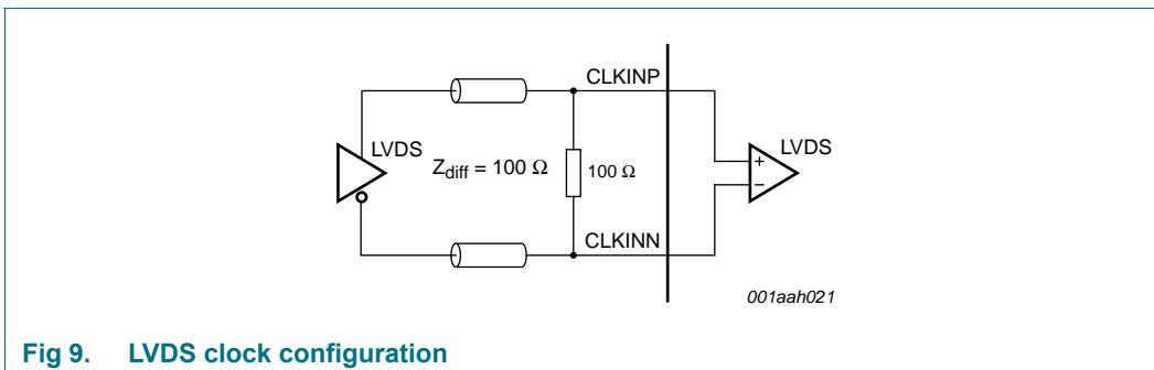
Fig 9. LVDS clock configuration
