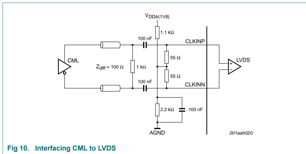
**Fig 10. Interfacing CML to LVDS**
