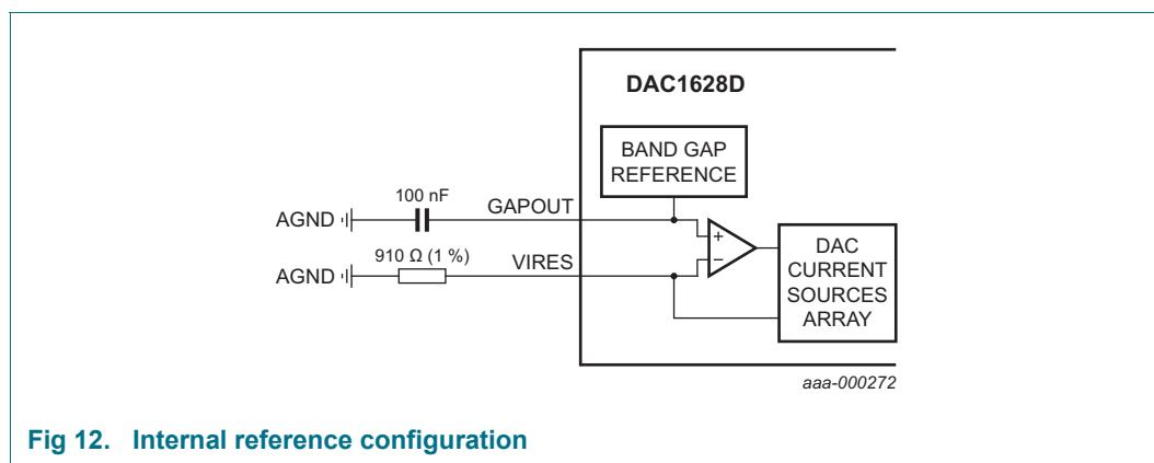
Figure 12 shows the optimal configuration for temperature drift compensation because the band gap reference voltage can be matched to the voltage across the feedback resistor.
