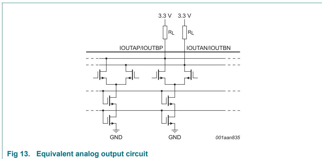
**Fig 13.** Equivalent analog output circuit
