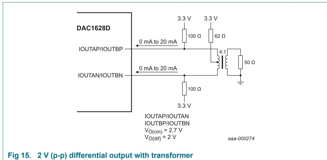
**Fig 15.** 2 V (p-p) differential output with transformer
