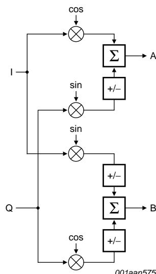
**Fig 11. Single-side band modulator principle**
