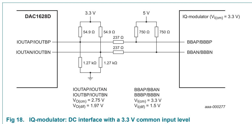
**Fig 18. IQ-modulator: DC interface with a 3.3 V common input level**
