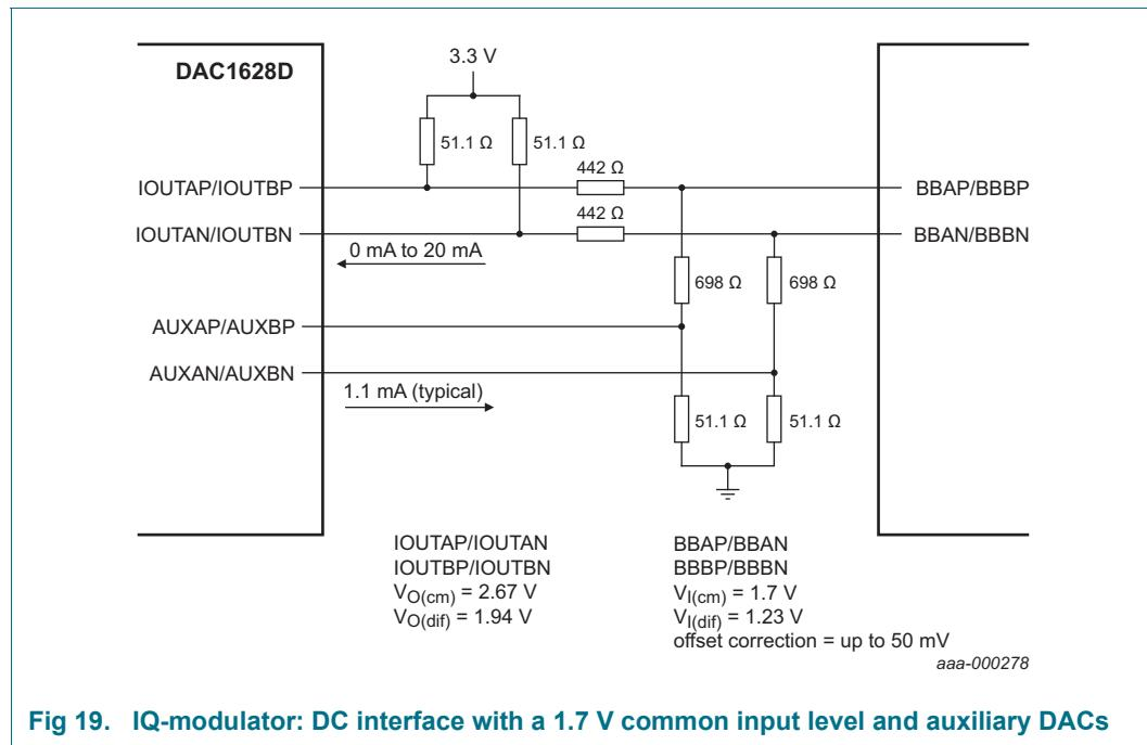
**Fig 19. IQ-modulator: DC interface with a 1.7 V common input level and auxiliary DACs**
