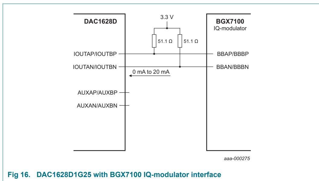
**Fig 16.** DAC1628D1G25 with BGX7100 IQ-modulator interface
