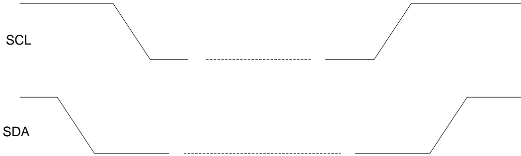
Figure 16: I 2 C START and STOP Condition Timing
