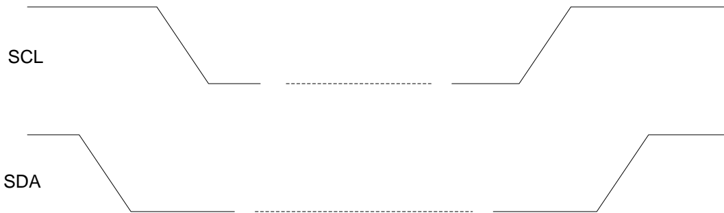
Figure 16: I 2 C START and STOP Condition Timing
