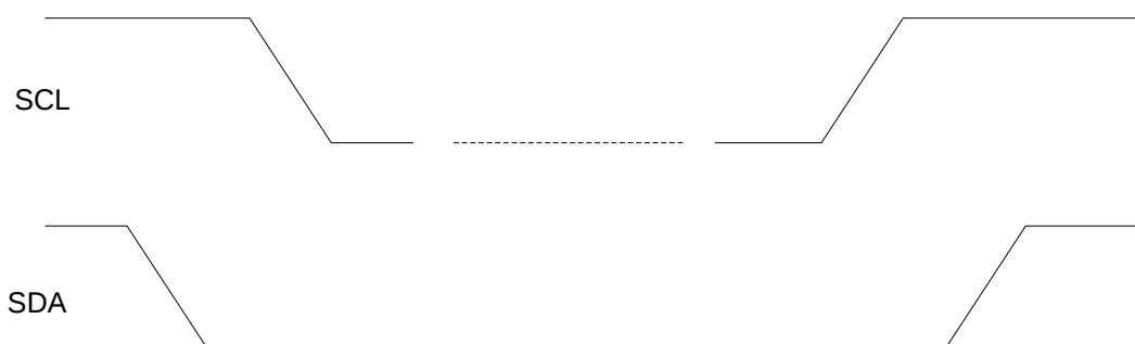
Figure 11. I 2 C START and STOP Condition Timing
