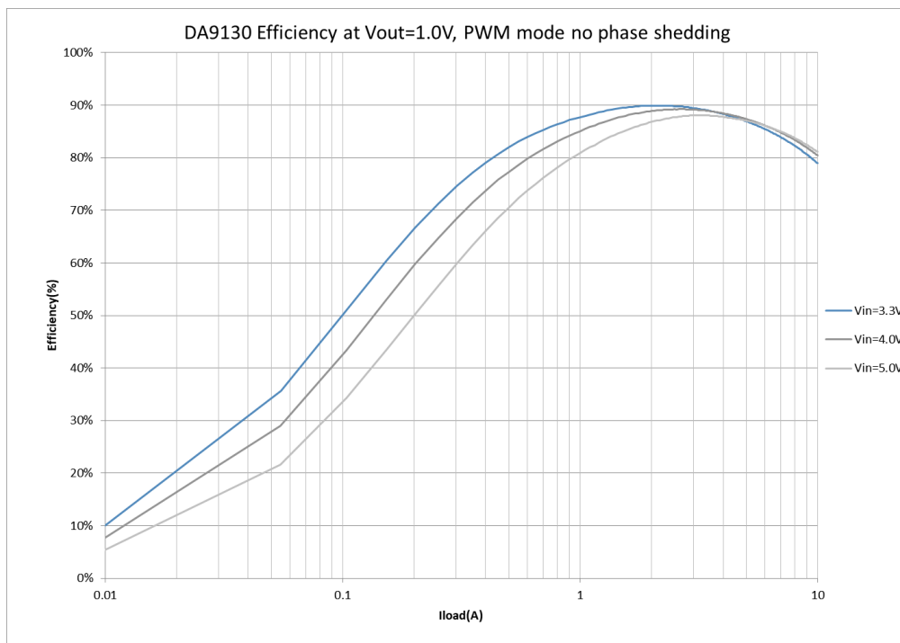
Figure 6. DA9130-A Efficiency, PWM Mode with no Phase Shedding
