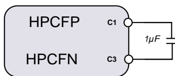
Figure 42. Charge pump flying capacitor
