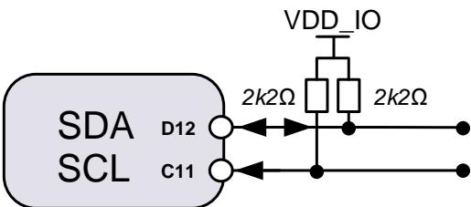
Figure 44. I<sup>2</sup>C pull upsTable 270: Digital interfaces – I<sup>2</sup>S
