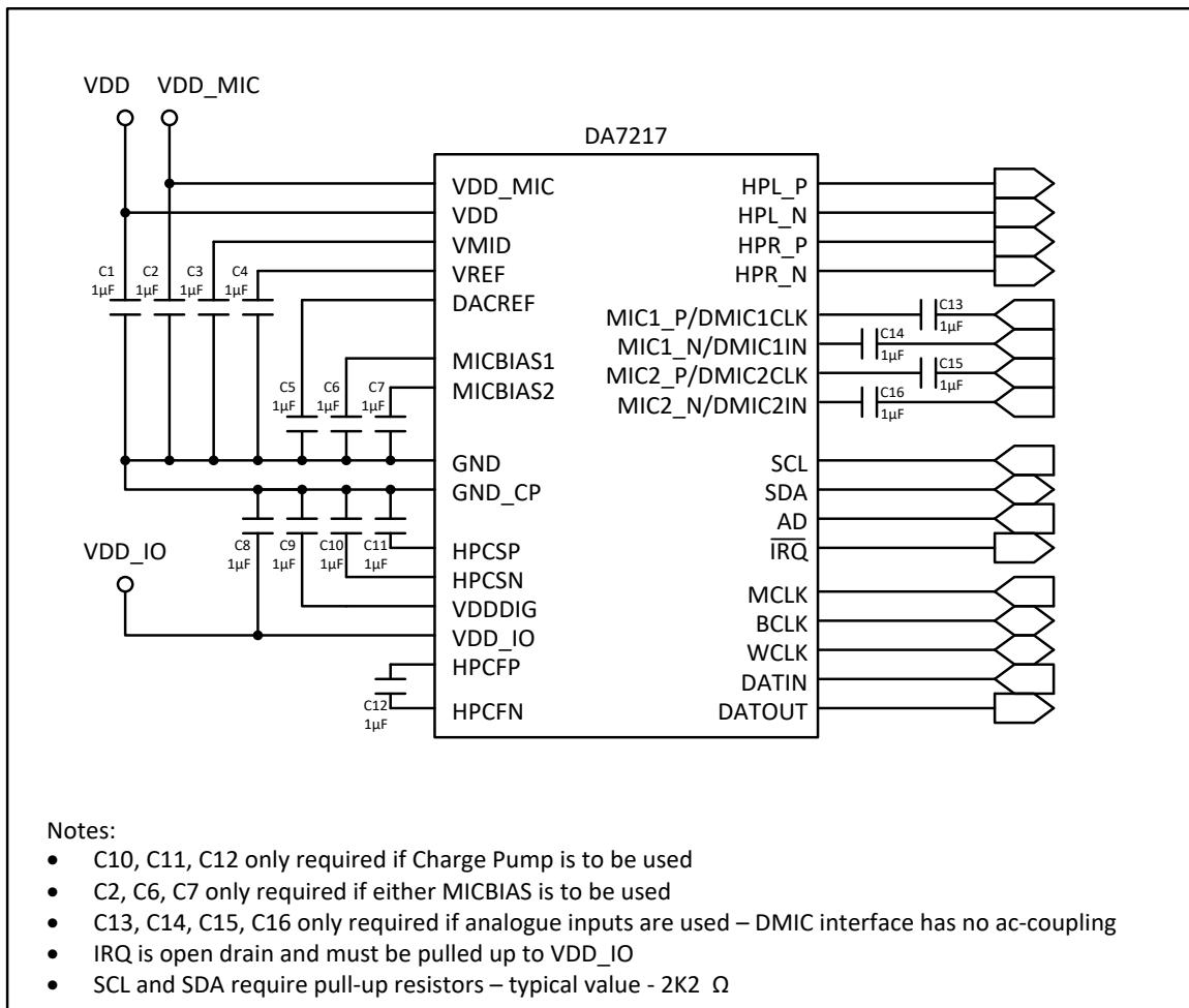
Figure 38. DA7217 external component requirements
