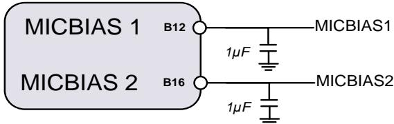
Figure 39. MICBIAS decoupling
