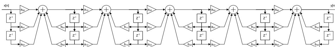
Figure 22. Cascade of five biquad filter stages
