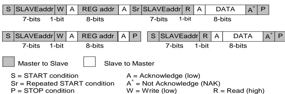
**Figure 28. Examples of the I<sup>2</sup>C byte read (SDA line)**
