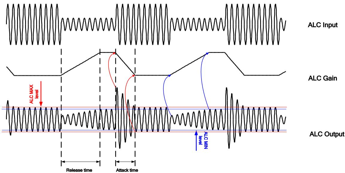
**Figure 11. Principle of operation of the ALC**
