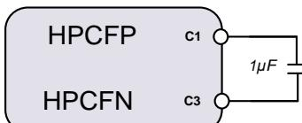
Figure 42. Charge pump flying capacitor
