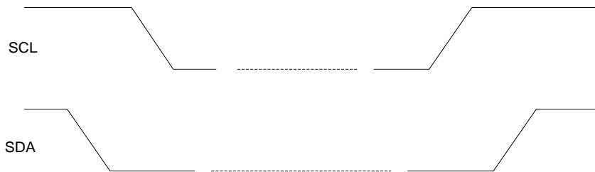
**Figure 26. Timing of I<sup>2</sup>C START and STOP conditions**
