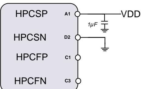
Figure 43. Single supply mode operation
