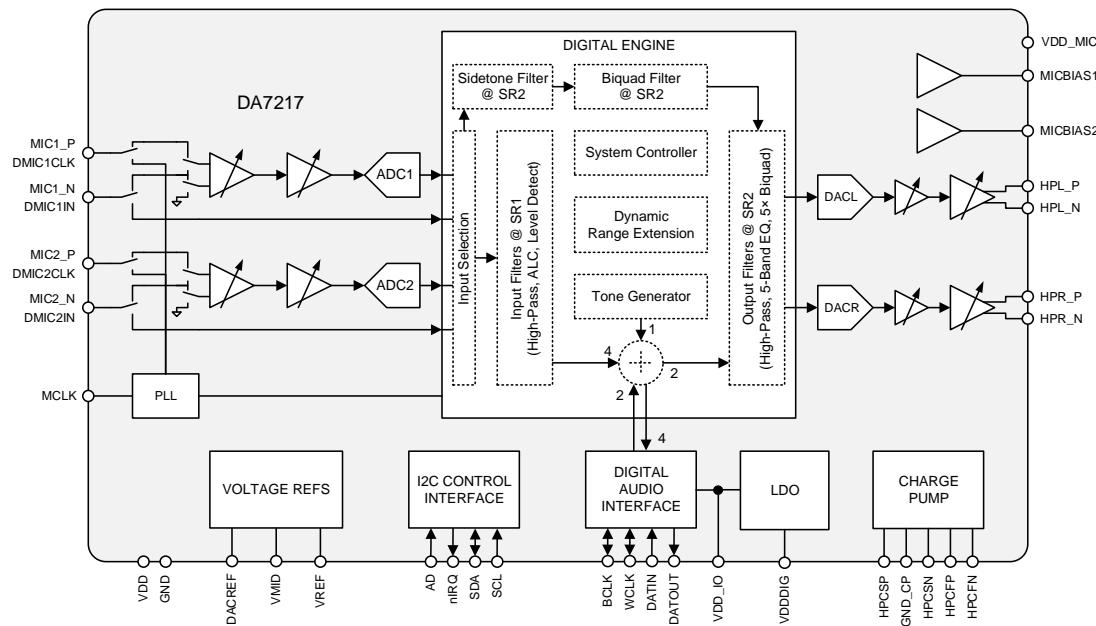
Figure 2. DA7217 block diagram
