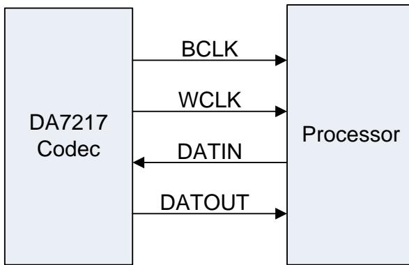
Figure 32. Master mode ([dai\\_clk\\_en = 1](#))
