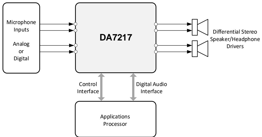
Figure 1. DA7217 with differential stereo headphone outputs
