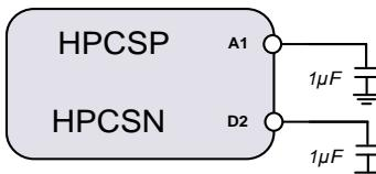
Figure 41. Charge pump decoupling
