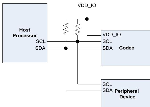
**Figure 25. Schematic of the I<sup>2</sup>C control interface bus**
