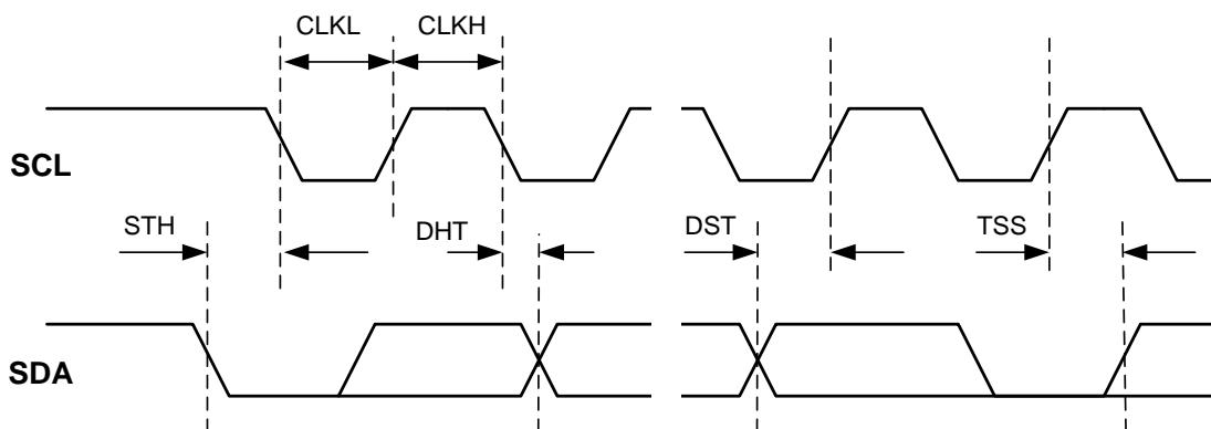
Figure 5. I<sup>2</sup>C bus timingTable 23: I<sup>2</sup>C control bus ( $V_{DD\_IO} = 1.8 \text{ V}$ )
