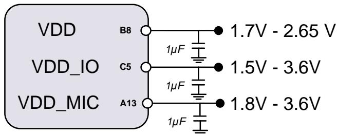
Figure 46. Power supply decoupling
