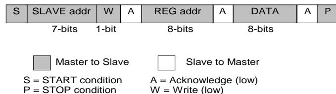
**Figure 27. I<sup>2</sup>C byte write (SDA signal)**
