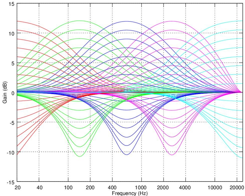
Figure 4. 5-Band equalizer response at 48 kHz
