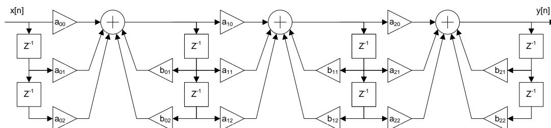
**Figure 14. Cascade of three biquad filter stages**
