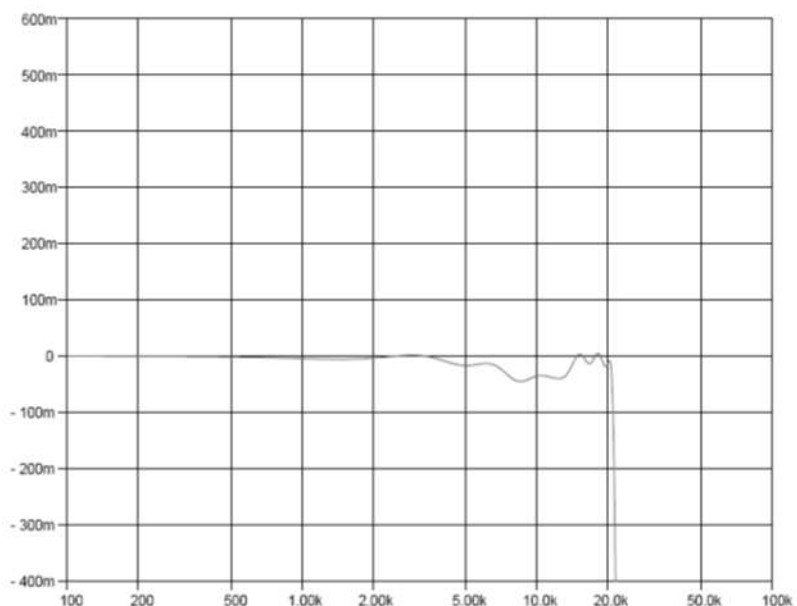
Figure 13: DAC Pass Band Attenuation (Audio Mode, 48 kHz)
