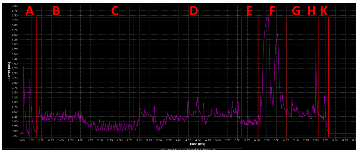
Figure 122: BLE Connection power profile
