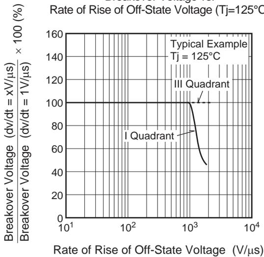
Breakover Voltage vs. Rate of Rise of Off-State Voltage ( $T_j=150^{\circ}C$ )
