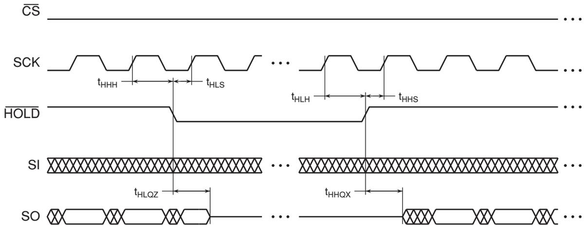
Figure 42.  $\overline{\text{HOLD}}$  Timing – Serial Output
