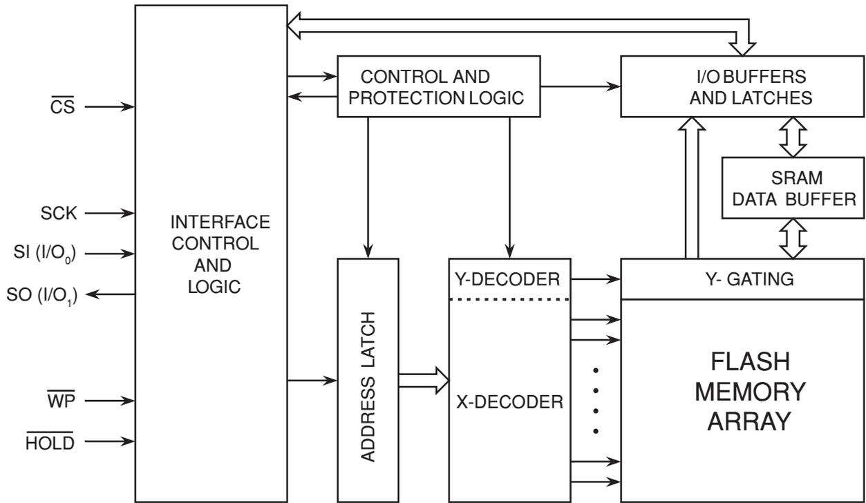
Figure 5. Block Diagram
