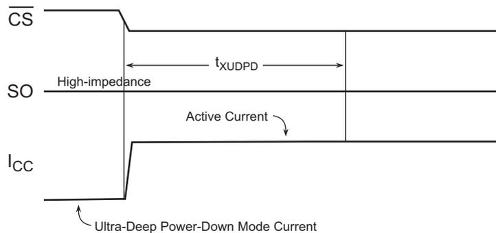
Figure 34. Exit Ultra-Deep Power-Down (Chip Select Low)
