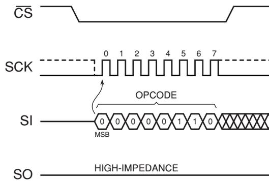
Figure 19. Write Enable
