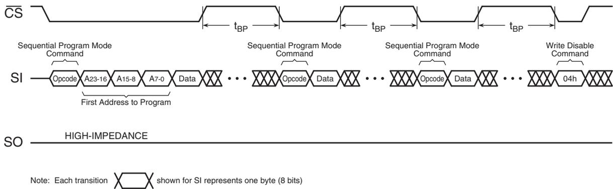
Figure 16. Sequential Program Mode – Waiting Maximum Byte Program Time
