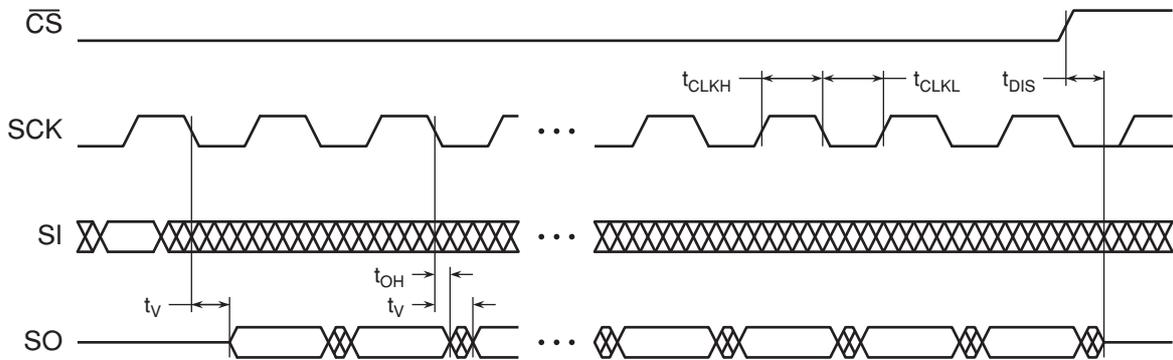
Figure 39. Serial Output Timing
