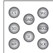
Figure 4. 8-ball WLCSP (Bottom View)
