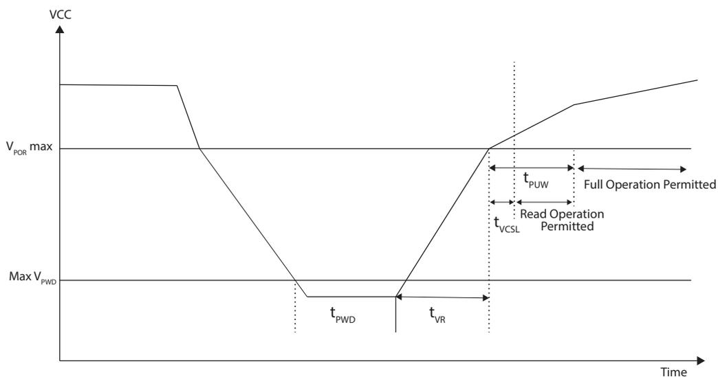
Figure 37. Power-Up Timing
