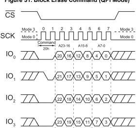
Figure 31. Block Erase Command (QPI Mode)
