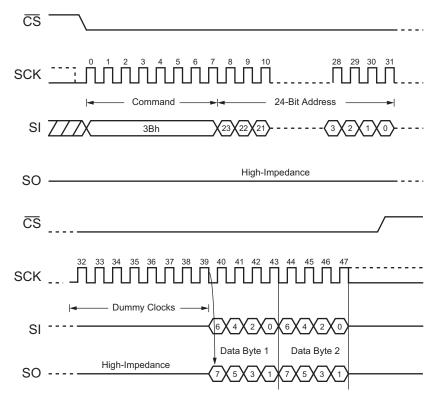
Figure 19. Fast Read Dual Output Command (SPI Mode)
