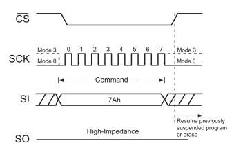
Figure 39. Erase / Program Resume Command (SPI Mode)
