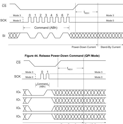
Figure 43. Release Power-Down Command (SPI Mode)
