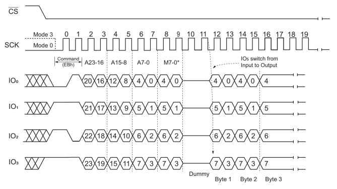
Figure 25. Fast Read Quad I/O Command (Initial command or previous M7-0 ≠ Axh, QPI mode)
