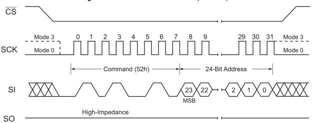
Figure 32. 32 kB Block Erase Command (SPI Mode)
