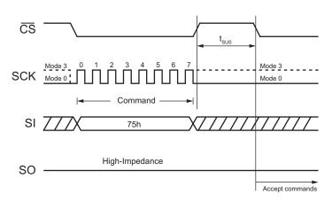
Figure 37. Erase Suspend Command (SPI Mode)
