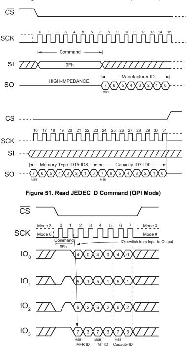
Figure 50. Read JEDEC ID Command (SPI Mode)
