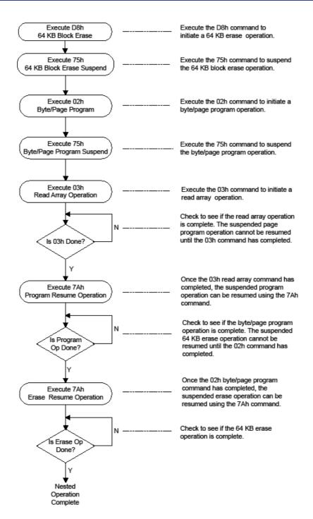
Figure 18. Flow Diagram of Nested Operations Example
