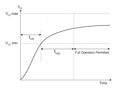
Figure 33. AC Timing During Device Power-Up
