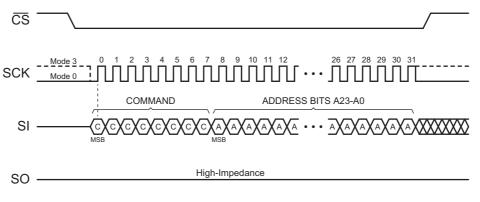
Figure 4. SPI Transfer — Command and Address Only
