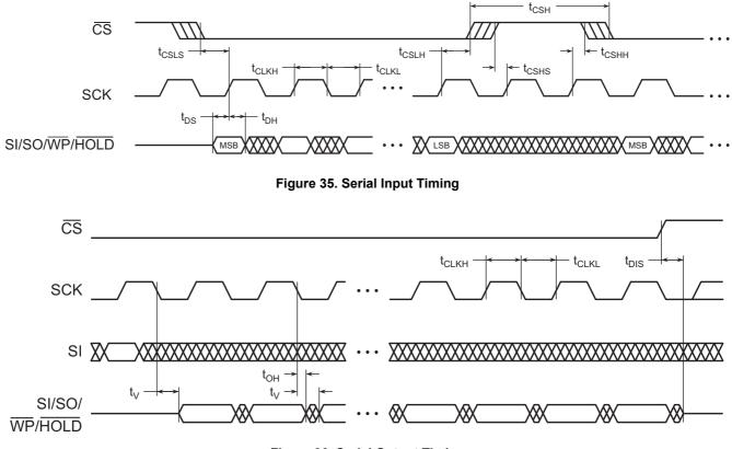
Figure 36. Serial Output Timing
