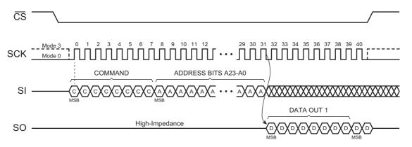
Figure 7. SPI Transfer — Command, Address, and Data — Read Operation with No Dummy Bytes
