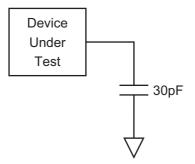
Figure 32. Output Test Load
