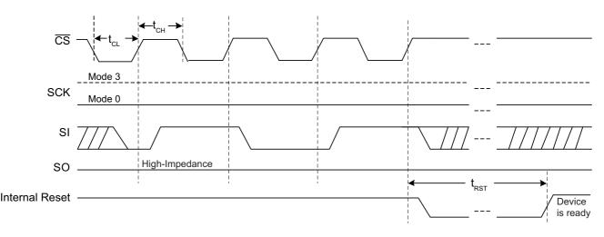
Figure 22. JEDEC Standard Hardware Reset
