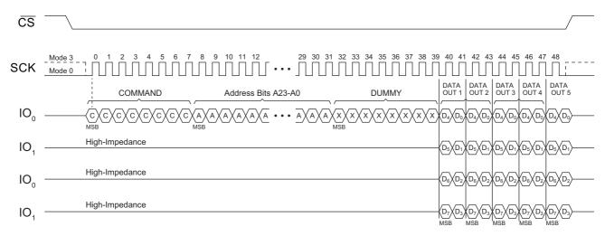
Figure 12. Quad Output Transfer — 1-Pin Command, 1-Pin Address, and 4-Pin Data — Read Operation
