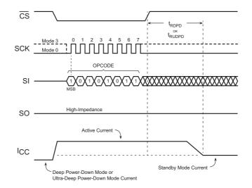
Figure 27. Resume from Deep Power-Down or Ultra-Deep Power-Down
