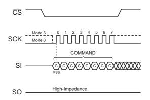
Figure 3. SPI Transfer — Command Only
