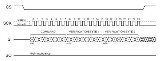
Figure 26. Status Register Lock Operation with Two Verification Bytes
