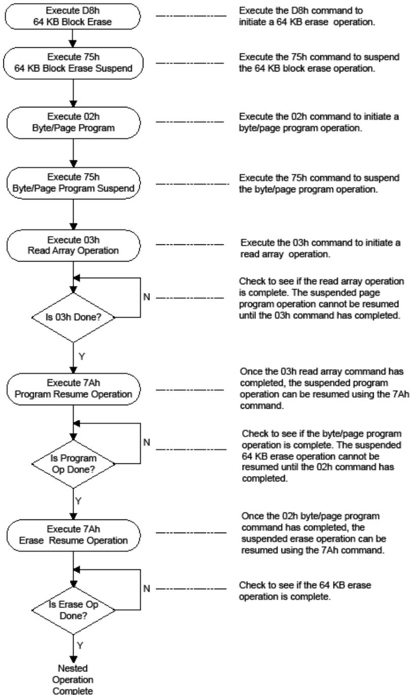
Figure 18. Flow Diagram of Nested Operations Example
