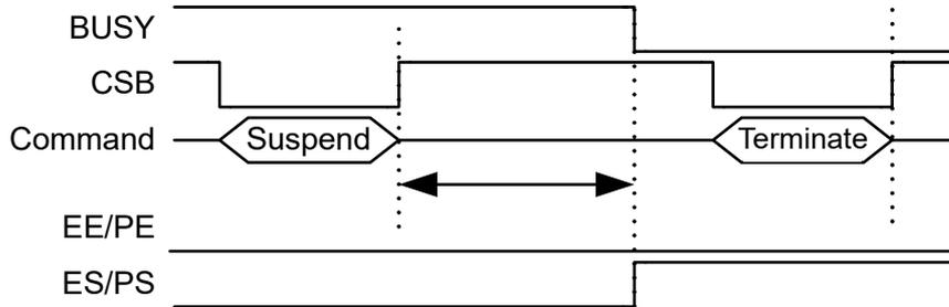
**Figure 20. Allowing Enough Time for the Suspend Operation to Complete**
