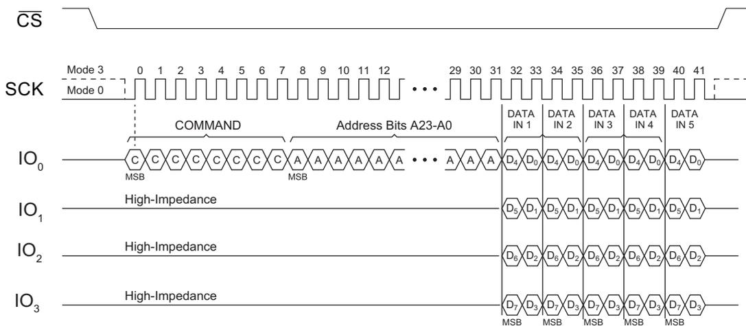
Figure 13. Quad Output Transfer — 1-Pin Command, 1-Pin Address, and 4-Pin Data — Write Operation
