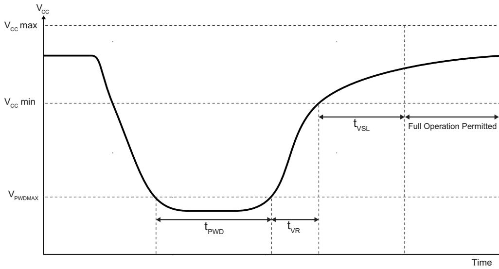
Figure 32. AC Power-up Timing After a Brown-Out
