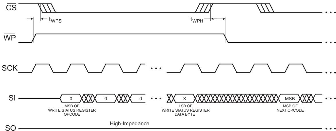
Figure 37.  $\overline{WP}$  Timing for Write Status Register Command
