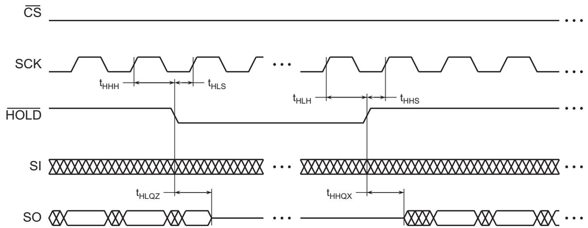
Figure 39.  $\overline{\text{HOLD}}$  Timing - Serial Output
