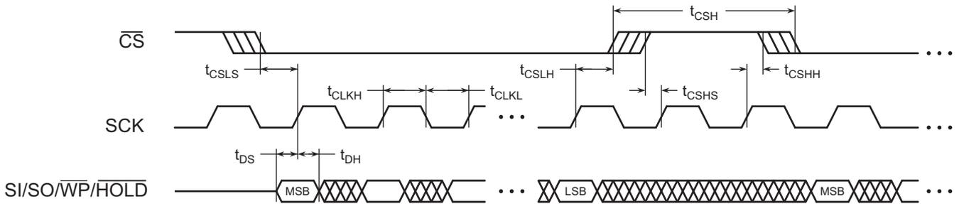
Figure 35. Serial Input Timing
