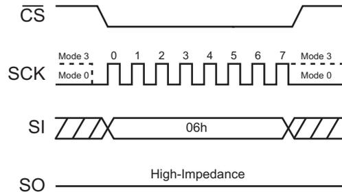
Figure 5. Write Enable Command for SPI Mode
