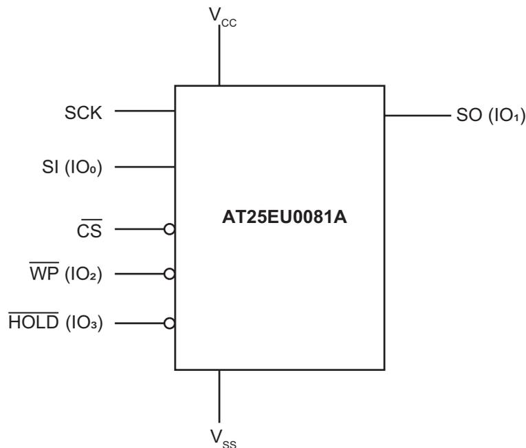
Figure 1. AT25EU0081A Logic Diagram
