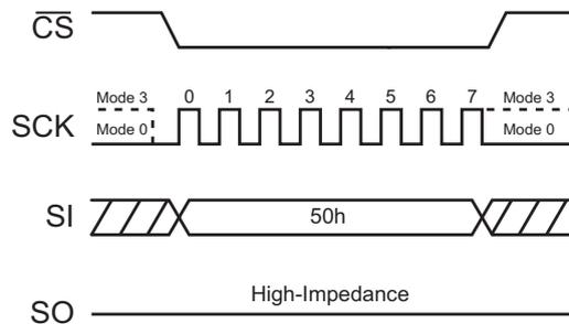
Figure 6. Write Enable for Volatile Status Register (50h)
