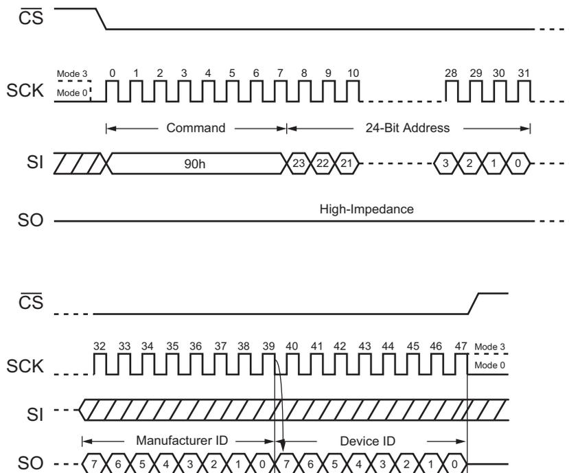
Figure 22. Read Manufacturer / Device ID Command
