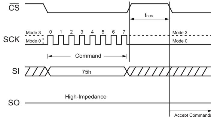
**Figure 36. Program/Erase Suspend Command**
