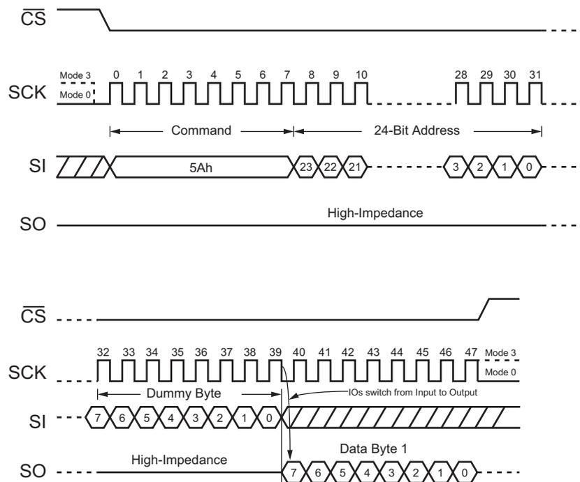
Figure 42. Read Serial Flash Discoverable Parameter Command
