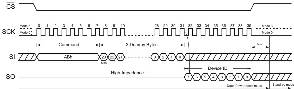
Figure 21. Release Power-Down / Device ID Command
