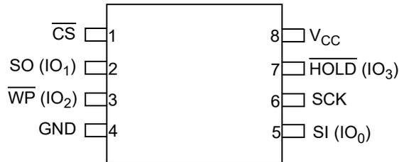
Figure 2. AT25EU0081A Pin Assignments, Eight-pin SOP 150-mil and 208-mil (Top View)
