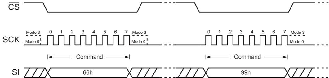
Figure 41. Enable Reset and Reset Command Sequence
