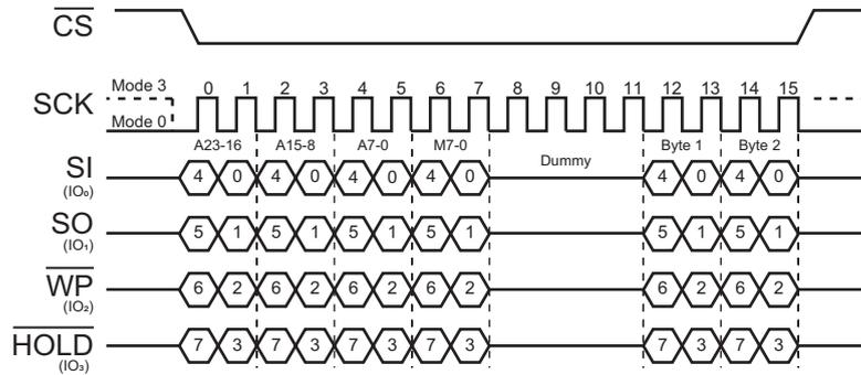
Figure 18. Fast Read Quad I/O Command (Previous command set M5-4=10)
