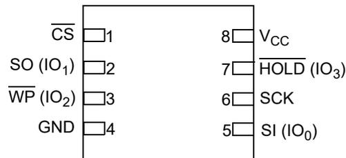
Figure 3. AT25EU0081A Pad Assignments, Eight-pad UDFN 2x3 mm (Top View)
