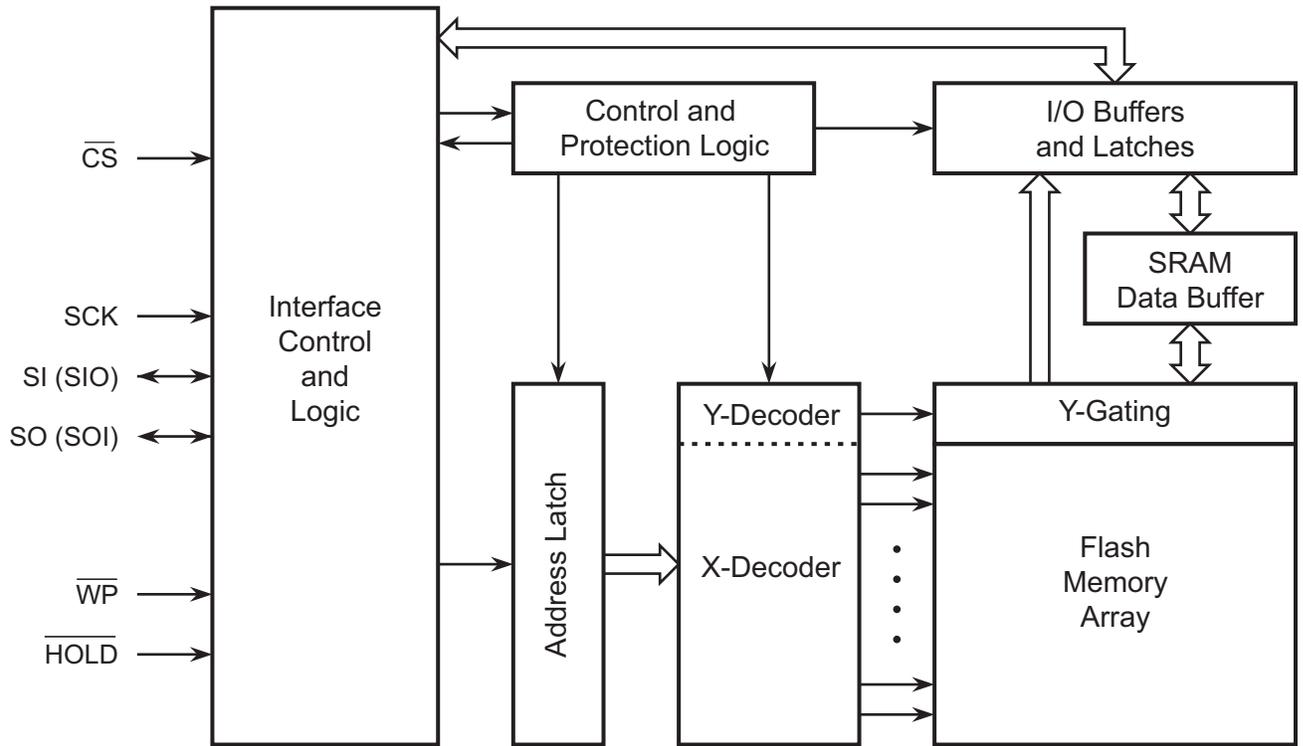
Note: SIO and SOI pin naming convention is used for Dual-I/O commands.
