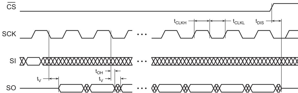
Figure 15-3.  $\overline{\text{WP}}$  Timing for Write Status Register Byte 1 Command When  $\text{SPRL} = 1$
