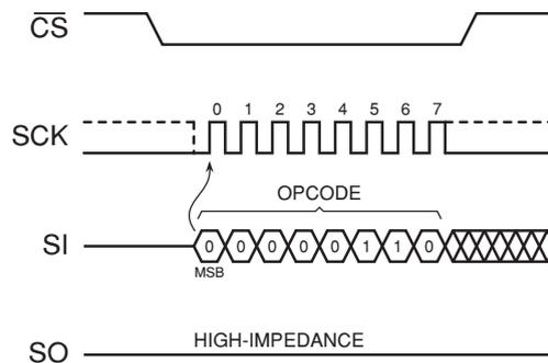
Figure 14. Write Enable
