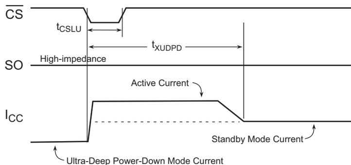
Figure 26. Exit Ultra-Deep Power-Down (Chip Select Toggle)
