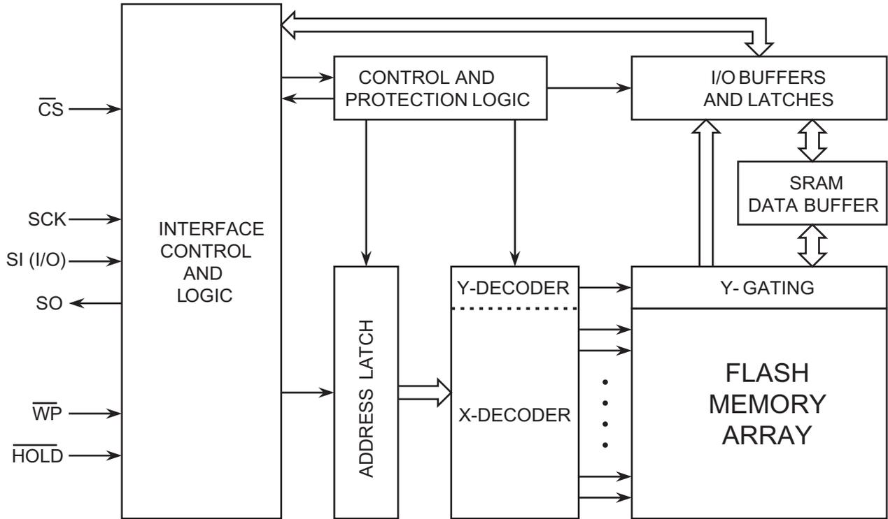
Figure 4. AT25DF011 Block Diagram
