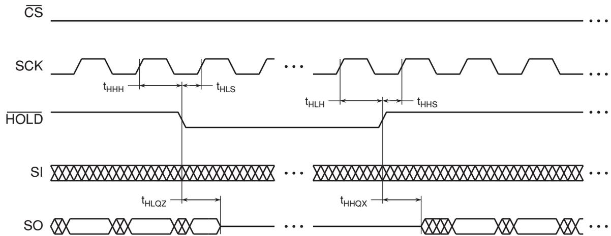
Figure 35.  $\overline{HOLD}$  Timing - Serial Output
