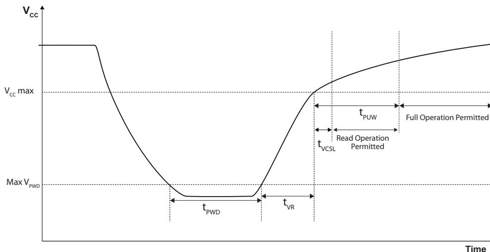
Figure 30. Power-Up Timing
