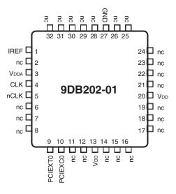
**32-Lead VFQFN**5mm x 5mm x 0.925 package body **K Package**Top View
