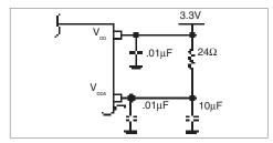
FIGURE 1. POWER SUPPLY FILTERING
