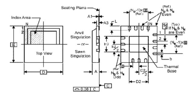
NOTE: The following package mechanical drawing is a generic drawing that applies to any pin count VFQFN package. This drawing is not intended to convey the actual pin count or pin layout of
