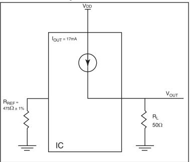
FIGURE 7. HCSL DRIVER CIRCUIT AND TERMINATION
