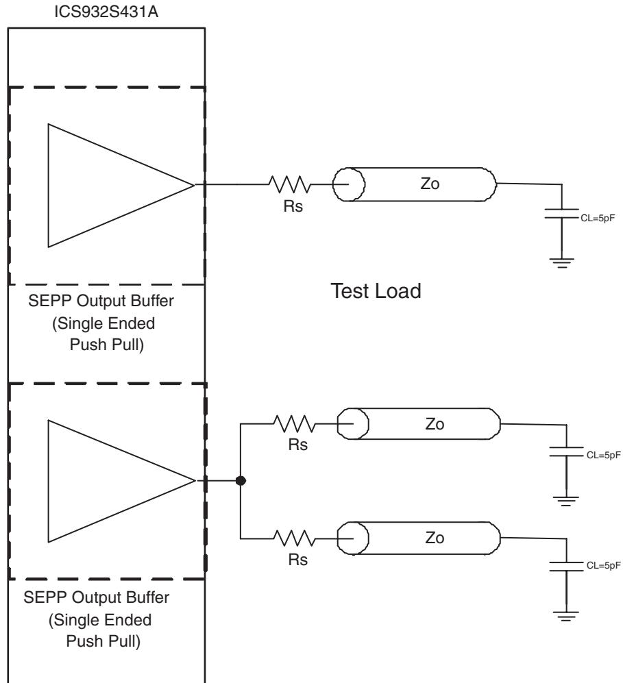
The singled-ended outputs of the ICS 932S4231A default to a drive strength of 2 loads. The REF clocks can be turned down to 1-load strength via the SMBus.
