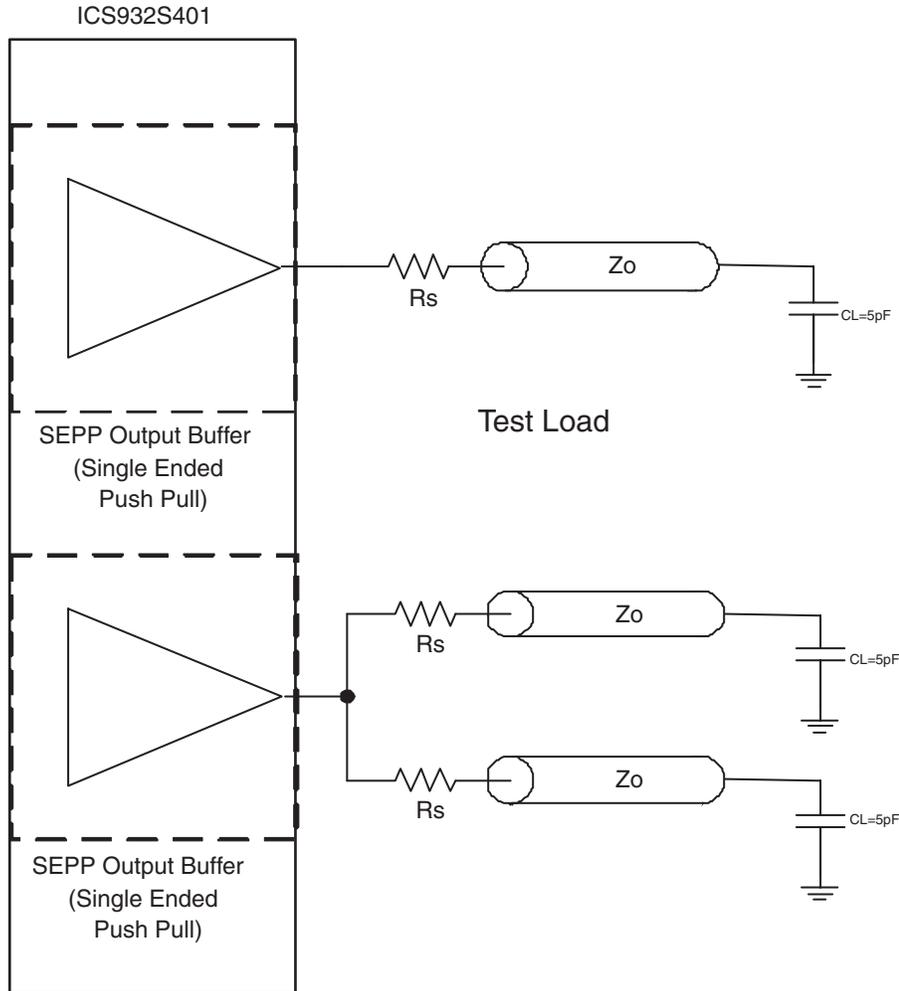
The singled-ended outputs of the ICS 932S401E default to a drive strength of 2 loads. The REF clocks can be turned down to 1-load strength via the SMBus. Suggested termination resistors are as follows for transmission lines with  $Z_o = 50$  ohms:
