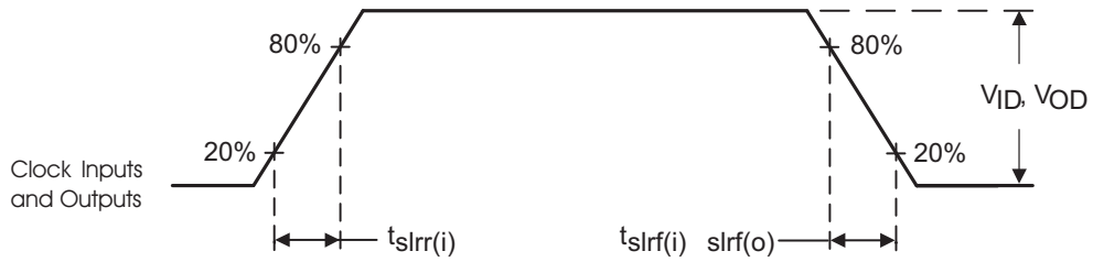
Figure 8. Input and Output Slew Rates
