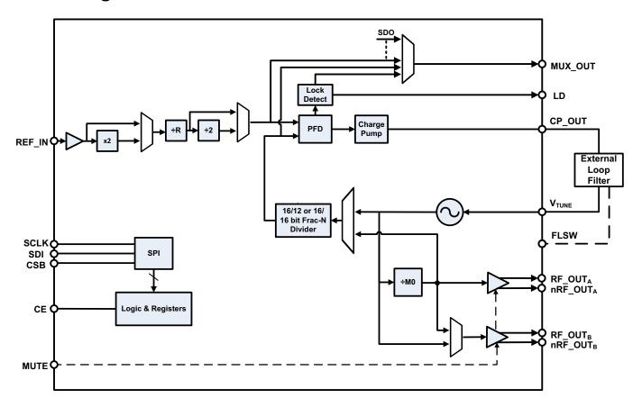
Note: 16-Bit Integer / 16-Bit Fractional feedback divider is available when using Register 6.
