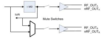
RF\_OUT and nRF\_OUT are derived from the drain of an NMOS differential pair driven by the VCO output (or by the M0 Divider), as shown in Figure 5.
