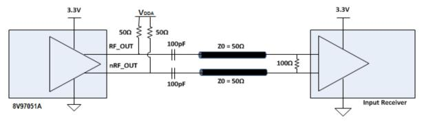
This termination scheme allows to provide one of the selected output power on the differential pair when connected to a  $50\Omega$  load. (See the RF Output Power for more information about the output power selection).
