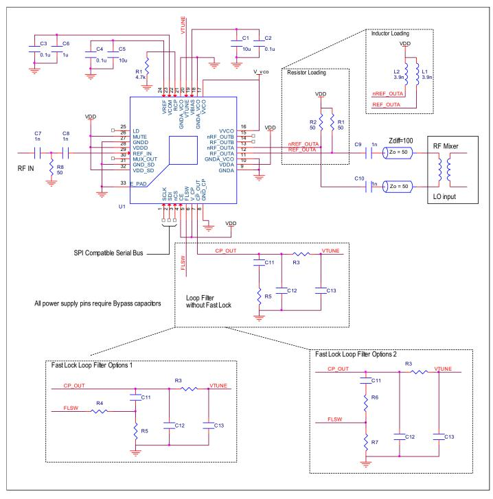
The 8V97051A output pull-up loading can be resistors or inductors. The pull up resistor value is typically  $50\Omega$ . Resistor pull up loading covers wide range of output frequencies. For inductor pull up loading, the inductor value is frequency dependent. One inductor value cannot cover all the output frequency range. This example shows the L = 3.9nH that is suitable for approximately 2GHz operating frequency. The output can also drive single ended LO input.
