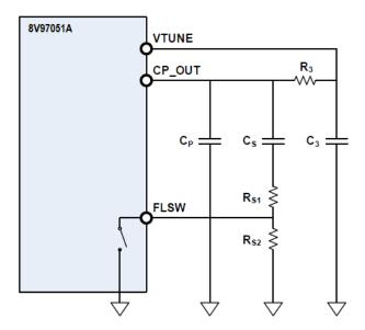
In the example of Figure 9, the damping resistor RS is equal to: RS1 + RS2 in normal mode (FSLW switch OFF), with RS2 = 3 \* RS1
