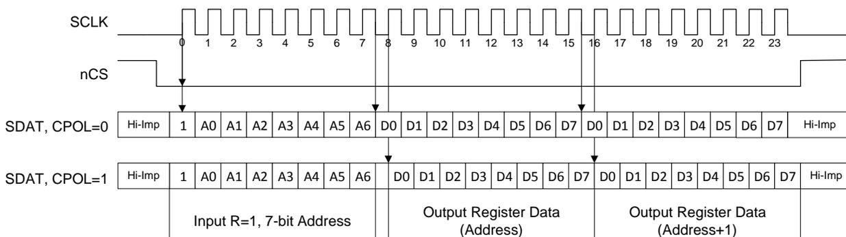
Figure 6. Logic Diagram: WRITE Data into Registers
