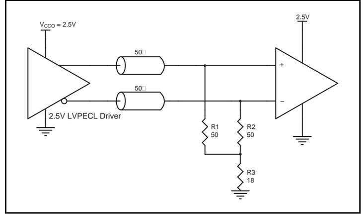
Figure 14C. 2.5V LVPECL Driver Termination Example
