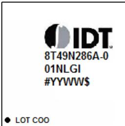
1. Line 1 and Line 2 indicate the part number. "001" will vary due to configuration.
