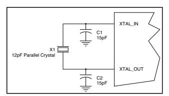
Figure 2. Crystal Input Interface
