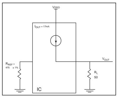
Figure 13. HCSL Driver Circuit and Termination
