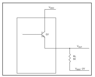
Figure 12. LVPECL Driver Circuit and Termination
