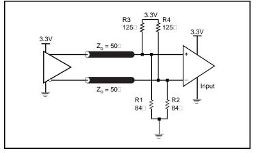
Figure 8B. 3.3V LVPECL Output Termination
