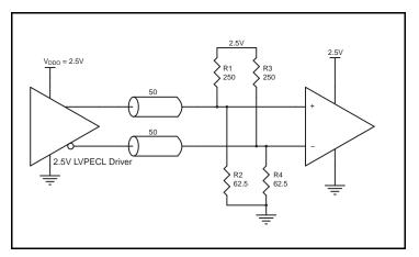
Figure 9A. 2.5V LVPECL Driver Termination Example
