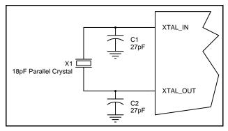
Figure 1. Crystal Input Interface
