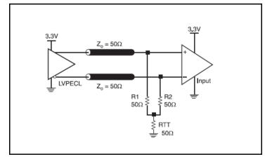
Figure 8A. 3.3V LVPECL Output Termination
