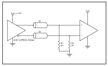
Figure 9C. 2.5V LVPECL Driver Termination Example
