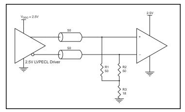
Figure 9B. 2.5V LVPECL Driver Termination Example
