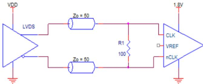
**Figure 5. Differential Input Driven by an LVDS Driver – AC Coupling**
