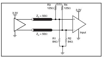
Figure 3B. 3.3V LVPECL Output Termination
