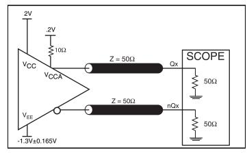
3.3V Output Load AC Test Circuit
