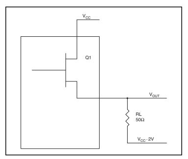
Figure 4. LVPECL Driver Circuit and Termination
