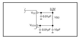
Figure 2. Power Supply Filtering
