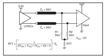
Figure 3A. 3.3V LVPECL Output Termination
