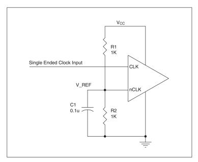
FIGURE 3. SINGLE ENDED SIGNAL DRIVING DIFFERENTIAL INPUT
