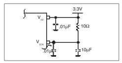
FIGURE 2. POWER SUPPLY FILTERING
