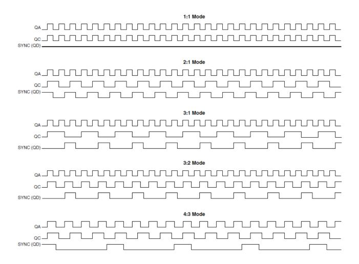
FIGURE 1. TIMING DIAGRAMS
