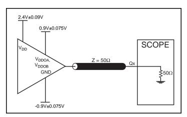
3.3V Core/1.8V Output Load AC Test Circuit
