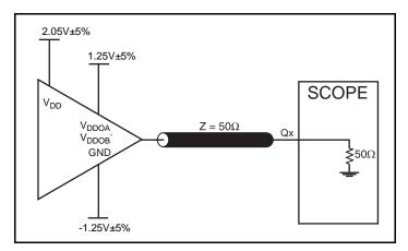
3.3V Core/2.5V Output Load AC Test Circuit
