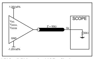
2.5V Core/2.5V Output Load AC Test Circuit
