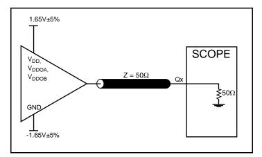
3.3V Core/3.3V Output Load AC Test Circuit
