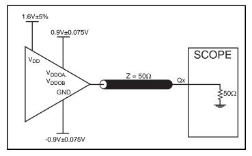
2.5V Core/1.8V Output Load AC Test Circuit
