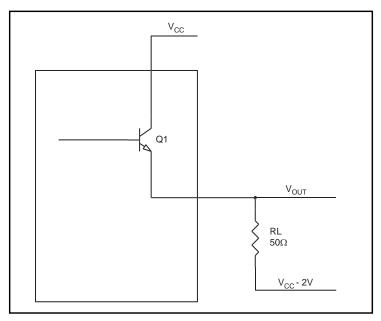
Figure 7. LVPECL Driver Circuit and Termination
