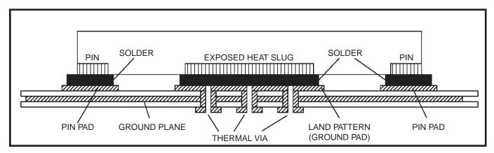
Figure 6. P.C. Assembly for Exposed Pad Thermal Release Path – Side View (drawing not to scale)
