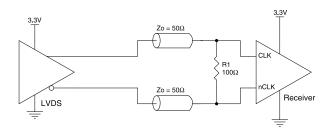
Figure 2D. CLK/nCLK Input Driven by a Built-In Pullup CML Driver
