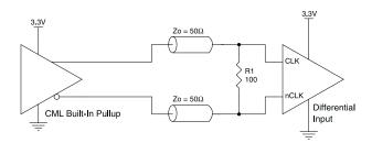
Figure 2E. CLK/nCLK Input Driven by an IDT Open Collector CML Driver
