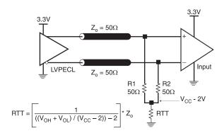
Figure 4B. 3.3V LVPECL Output Termination
