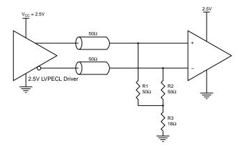
Figure 5C. 2.5V LVPECL Driver Termination Example
