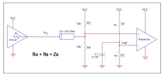
Figure 1. Recommended Schematic for Wiring a Differential Input to Accept Single-ended Levels
