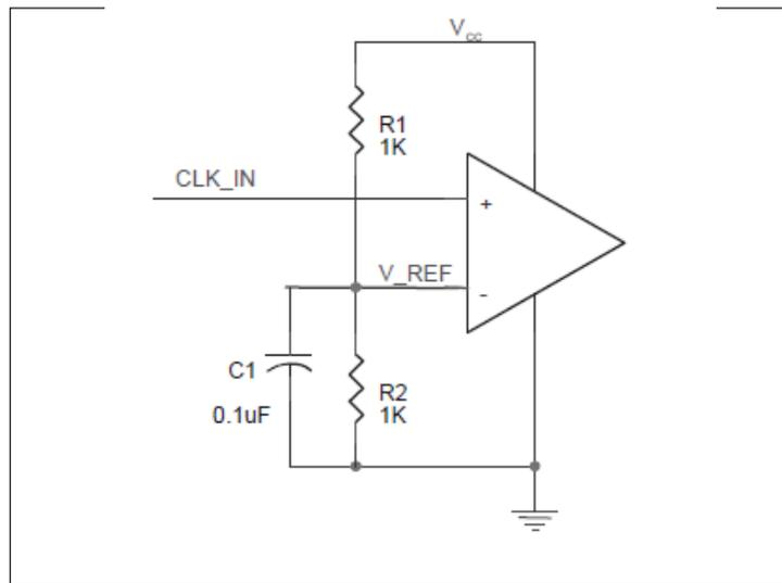
FIGURE 2. SINGLE ENDED SIGNAL DRIVING DIFFERENTIAL INPUT
