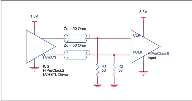
**FIGURE 3A. CLK/nCLK INPUT DRIVEN BY HSTL DRIVER**
