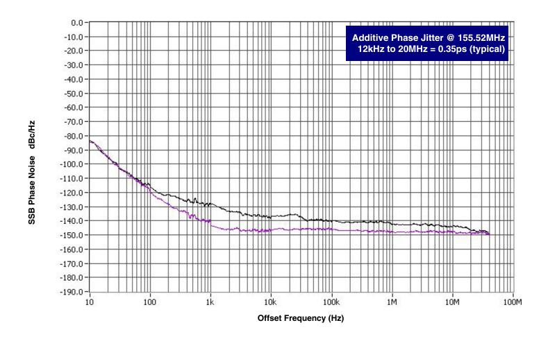
As with most timing specifications, phase noise measurements has issues relating to the limitations of the equipment. Often the noise floor of the equipment is higher than the noise floor of the device. This
