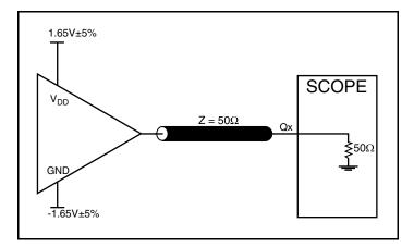
3.3V Output Load AC Test Circuit
