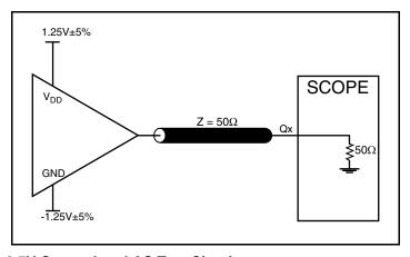
2.5V Output Load AC Test Circuit
