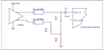
Figure 3B. General Diagram for LVPECL Driver to XTAL Input Interface
