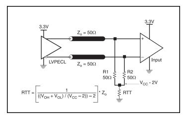
Figure 4A. 3.3V LVPECL Output Termination
