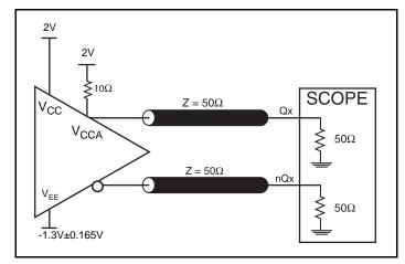
3.3V LVPECL Output Load AC Test Circuit
