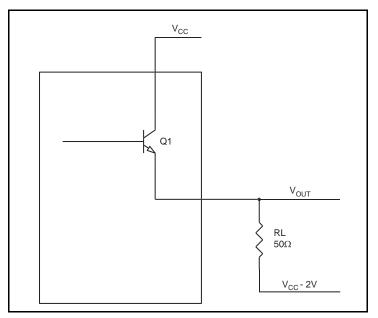
Figure 6. LVPECL Driver Circuit and Termination
