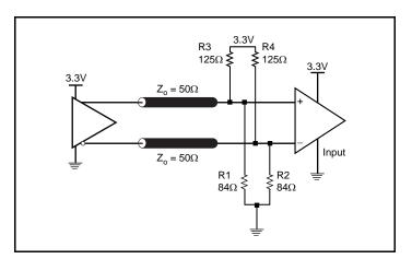
Figure 4B. 3.3V LVPECL Output Termination
