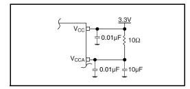
Figure 1. Power Supply Filtering
