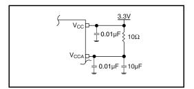
Figure 1. Power Supply Filtering
