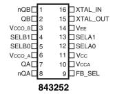
16-Lead TSSOP 4.4mm x 5.0mm x 0.925mm package body G Package
