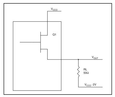
Figure 6. LVPECL Driver Circuit and Termination
