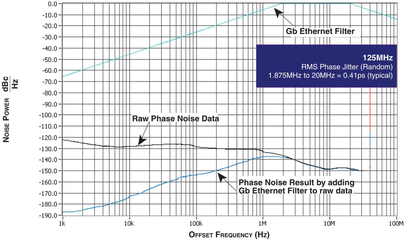
TYPICAL PHASE NOISE AT 312.5MHz @ 3.3V
