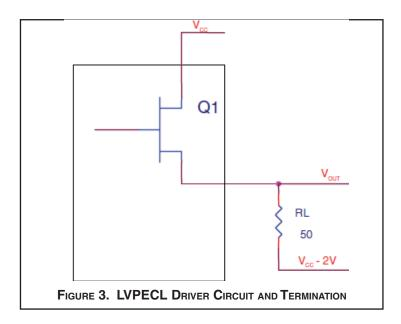
To calculate worst case power dissipation into the load, use the following equations which assume a  $50\Omega$  load, and a termination voltage of  $V_{cc}$ - 2V.
