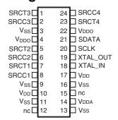
842S104E 24-Lead TSSOP 4.4mm x 7.8mm x 0.925mm package body G Package Top View
