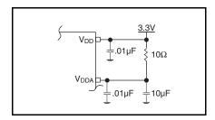
Figure 1. Power Supply Filtering
