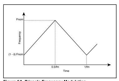
Figure 5A. Triangle Frequency Modulation
