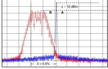
Figure 5B. 200MHz Clock Output In Frequency Domain
