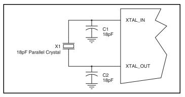
Figure 2. Crystal Input Interface
