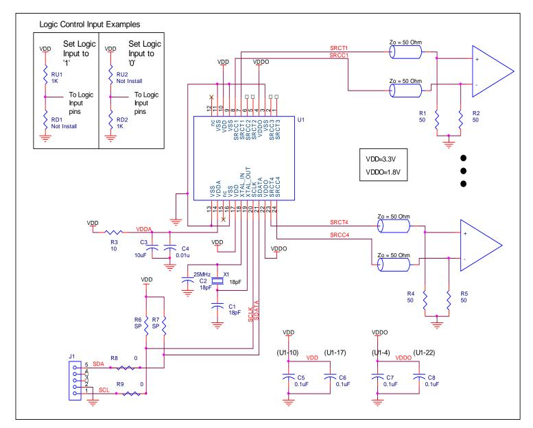
Figure 6. 842S104E Schematic Example
