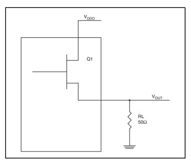
Figure 7. HSTL Driver Circuit and Termination
