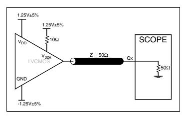
2.5V Output Load AC Test Circuit
