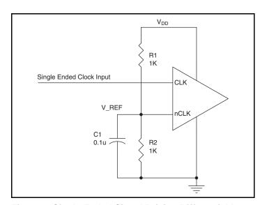
Figure 2. Single-Ended Signal Driving Differential Input
