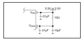
Figure 1. Power Supply Filtering
