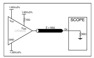
3.3V Output Load AC Test Circuit
