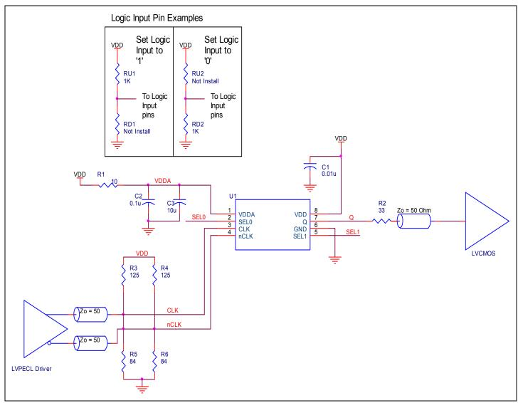
Figure 4. ICS840271I Schematic layout
