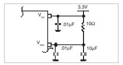
FIGURE 1. POWER SUPPLY FILTERING
