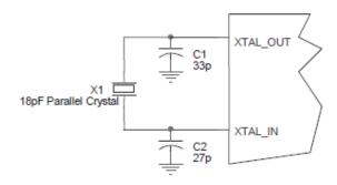
FIGURE 2. CRYSTAL INPUT INTERFACE
