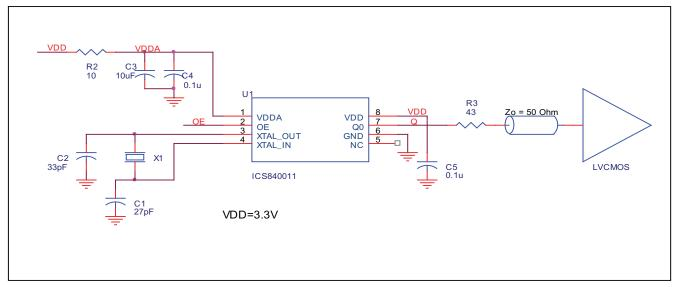
FIGURE 4A. 840011 SCHEMATIC EXAMPLE
