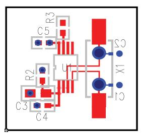
FIGURE 4B. 840011 PC BOARD LAYOUT EXAMPLE
