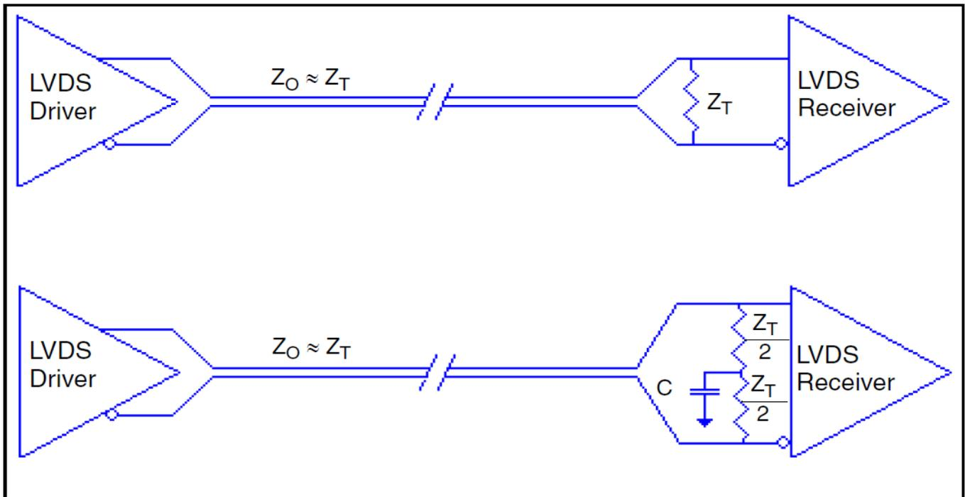
Figure 30. Recommended LVDS Output Port Line Termination
