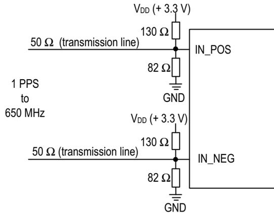
Figure 23. Recommended PECL Input Port Line Termination
