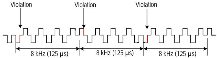
Figure 18. 64 kHz + 8 kHz Signal Structure
