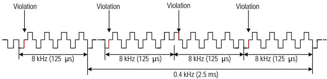
Figure 19. 64 kHz + 8 kHz + 0.4 kHz Signal Structure
