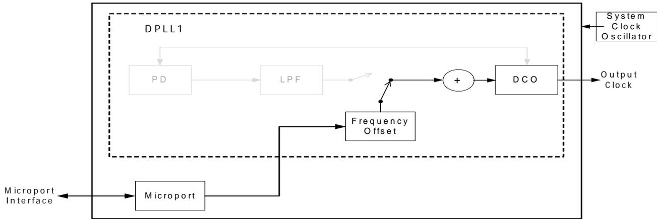
Figure 6. DCO frequency offset control functional block diagram
