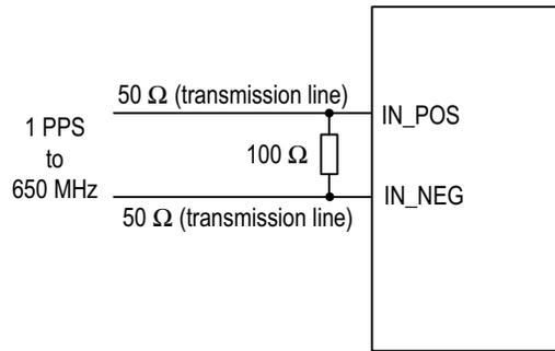
Figure 29. Recommended LVDS Input Port Line Termination
