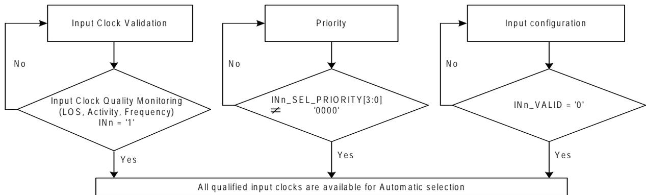
Figure 11. Qualified Input Clocks for Automatic Selection
