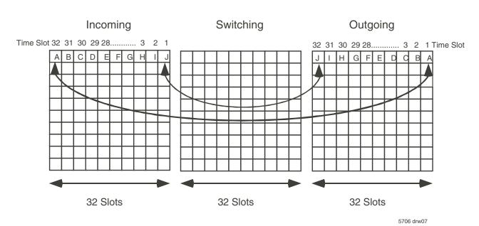
For Slot 1 ("A"): IN=32, OUT=1, DELAY=(32-32)+32+(1-1)=32 time slots minimum delay For Slot 32 ("J"): IN=1, OUT=32, DELAY=(32-1)+32+(32-1)=94 time slots maximum delay
