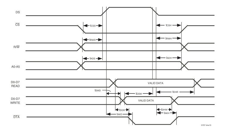
Figure 12. Motorola Non-Multiplexed Bus Timing
