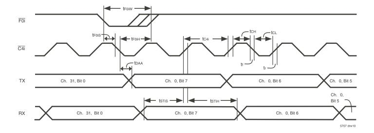
Figure 7. ST-BUS® Timing
