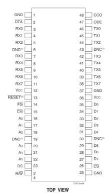
Package TypeReference IdentifierOrder CodeSSOP: 0.025in. pitch, 0.625in. x 0.295in.SO48-1PV
