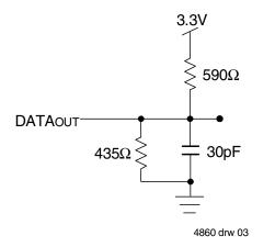
Figure 1. AC Output Test load.
