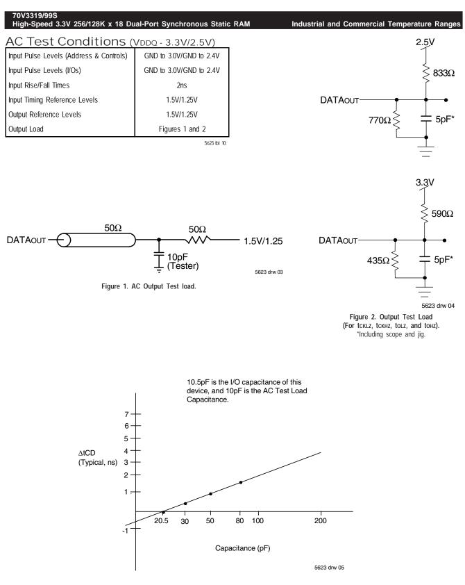
Figure 3. Typical Output Derating (Lumped Capacitive Load).
