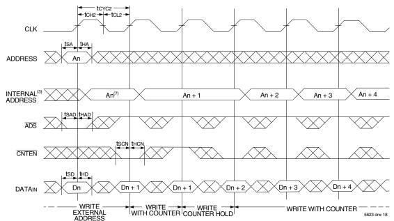
Timing Waveform of Counter Repeat<sup>(2)</sup>
