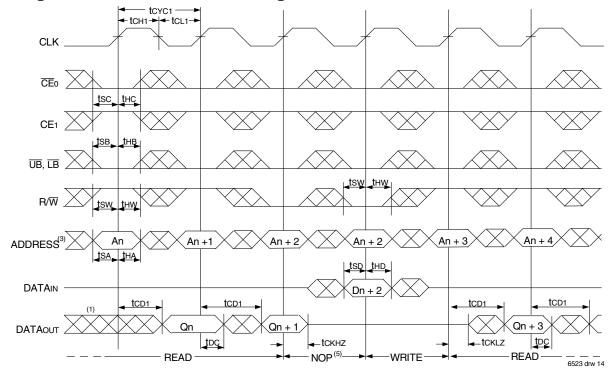
Timing Waveform of Flow-Through Read-to-Write-to-Read (**OE** Controlled)<sup>(2)</sup>
