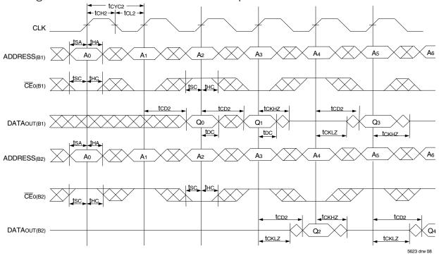
Timing Waveform of a Multi-Device Flow-Through Read<sup>(1,2)</sup>
