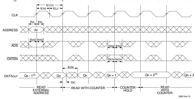
Timing Waveform of Flow-Through Read with Address Counter Advance<sup>(1)</sup>
