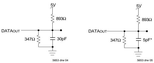
Figure 1. AC Output Test load.
