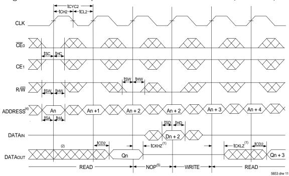
Timing Waveform of Pipelined Read-to-Write-to-Read (**OE** Controlled)(3)
