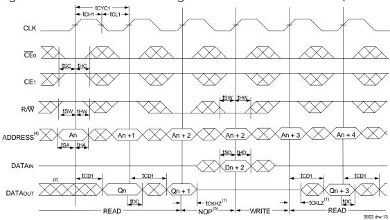
Timing Waveform of Flow-Through Read-to-Write-to-Read (**OE** Controlled)(3)
