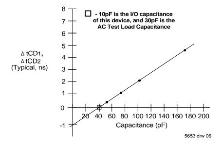
Figure 3. Typical Output Derating (Lumped Capacitive Load).
