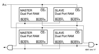
Figure 3. Busy and chip enable routing for both width and depth expansion with IDT7018 RAMs.
