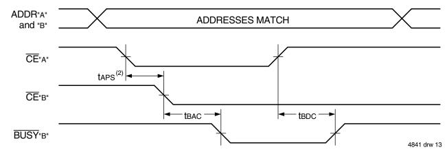
Waveform of **BUSY** Arbitration Cycle Controlled by Address Match Timing  $(M/S = VIH)^{(1)}$
