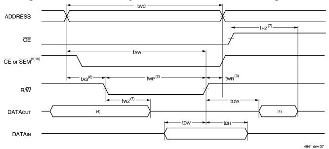
Timing Waveform of Write Cycle No. 2,  $\overline{CE}$  Controlled Timing<sup>(1,5)</sup>
