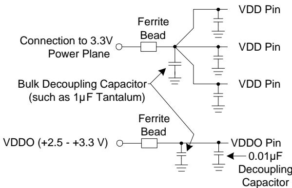
All power supply pins must be connected to the same voltage, except VDDO, which may be connected to a lower voltage in order to change the output level.
