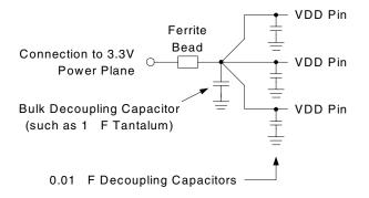
All power supply pins must be connected to the same voltage, except VDDR and VDDO, which may be connected to a lower voltage in order to change the output level. If the reference output is not used, ground VDDR.
