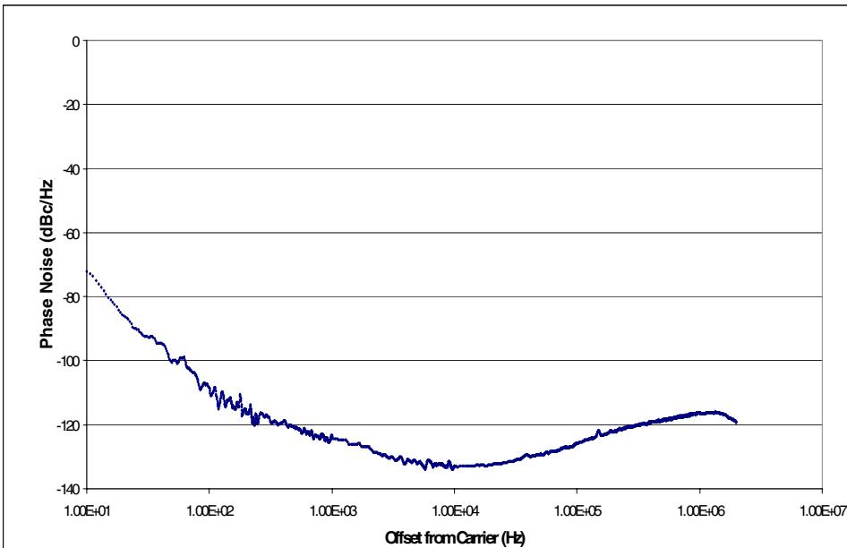
Figure 1. Phase Noise of ICS601-01 for 125 MHz output, 25 MHz crystal input.
