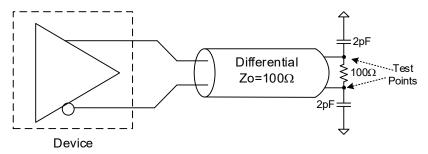
Figure 5. LVPECL Test Load
