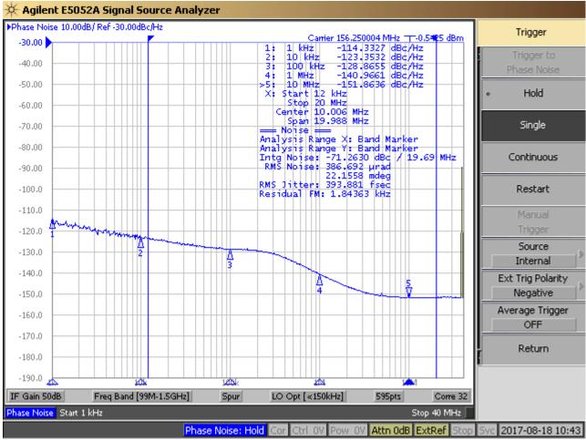
Note: Measured with OUT2=156.25MHz on, 39.625MHz input.
