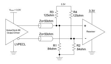
Figure 16. 2.5V LVPECL Output Termination (2)
