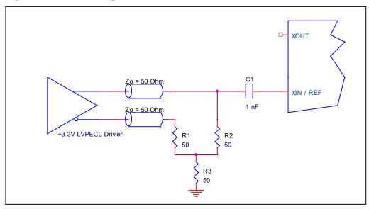
Table 23 shows resistor values that ensure the maximum drive level for the CLKIN port is not exceeded for all combinations of 5% tolerance on the driver  $V_{DD}$ ,  $V_{DDO0}$ , and 5% resistor tolerances. The resistor values can be adjusted to reduce the loading for a slower and weaker LVCMOS driver by increasing the impedance of the R1–R2 divider. To better assist with this assessment, the total load (Ro+Rs+R1+R2) on the driver is included in the table.
