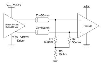
Figure 14. 3.3V LVPECL Output Termination (2)
